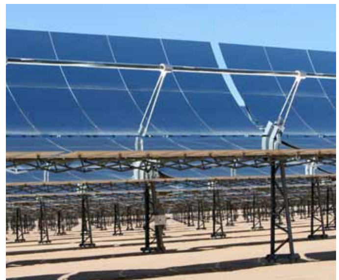
Illustration 3. Parabolic trough solar concentrators
