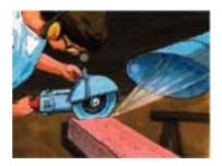
For certain activities, such as sharpening tools, cutting wood, polishing metals or using other mechanical hand tools, enterprises must provide individual protection equipment, such as safety goggles, gloves, etc., and must ensure that workers use them appropriately.
