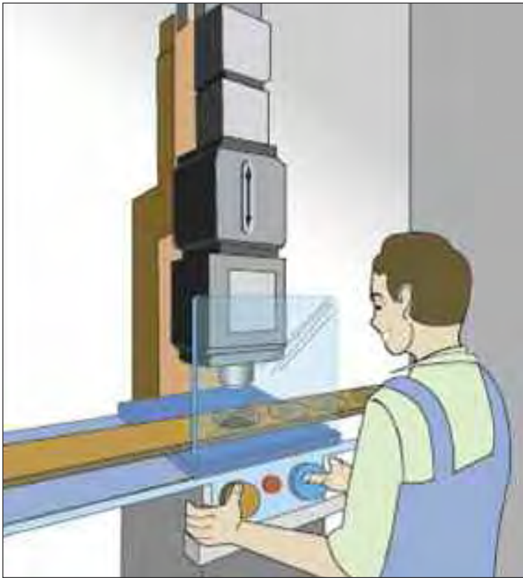
Figure 23a. Apply engineering controls, such as two-button control for a dangerous press machine, so that workers are not exposed to associated risks.
